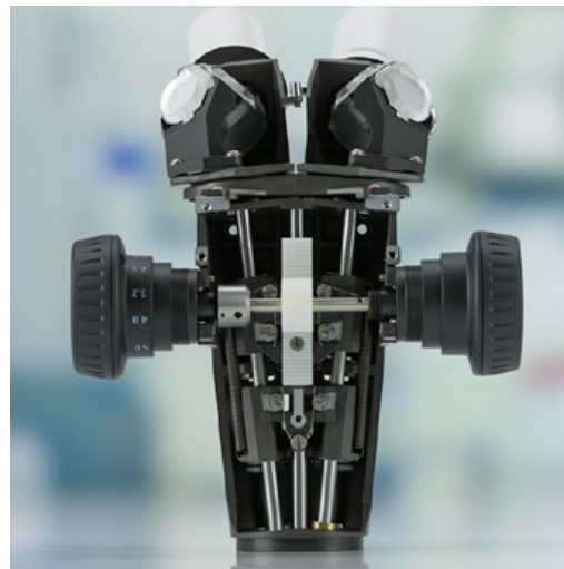
Stemi 508 is a Greenough type stereo microscope with twin body tubes, inclined by 11° – featuring a powerful 8:1 zoom
